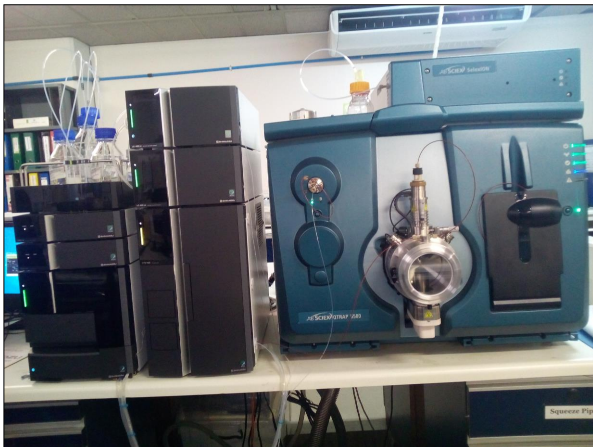
Figure 5: Shimadzu UPLC (Ultra Pressure Liquid Chromatography) coupled to Sciex QTrap 5500 Selextion mass spectrometer.
