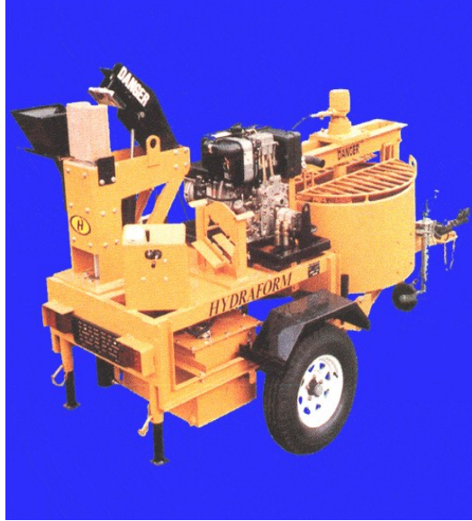
c) Hydraform mobile block making machine
