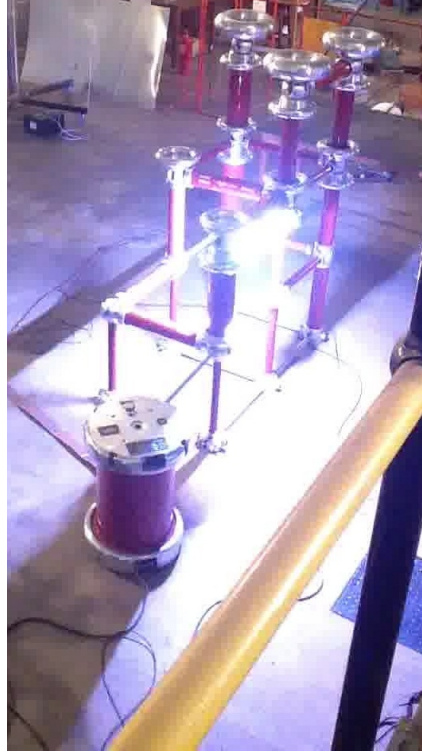
Figure 5.2: Still from a video of flashover over the circuit of the DC generator in the HV Lab at the University of the Witwatersrand
