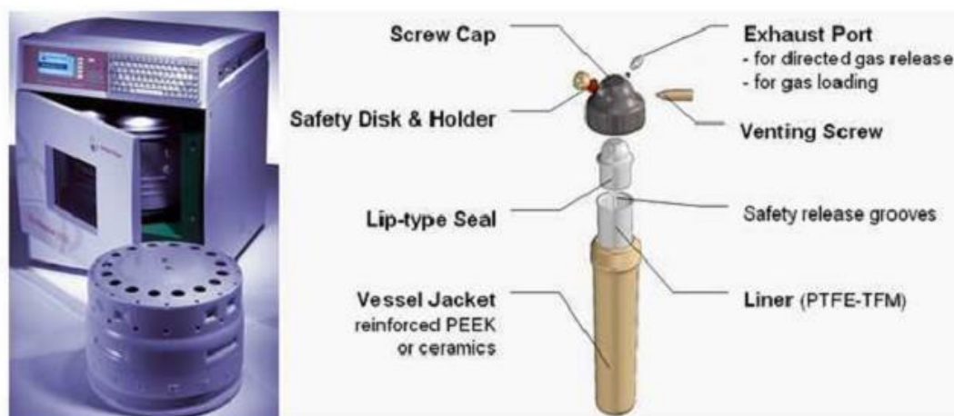
Figure 4.1: Anton Paar Multiwave 3000 microwave assisted extraction system (Multiwave 3000, Anton Paar, Graz, Austria).
