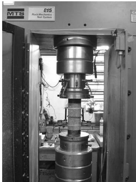
Figure 10: Uniaxial compression test equipment [16]
