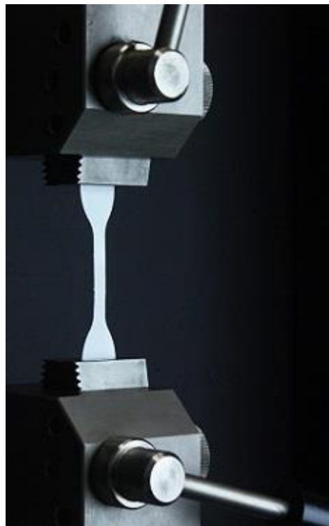
Figure 9: Uniaxial Tension Testing [14]
