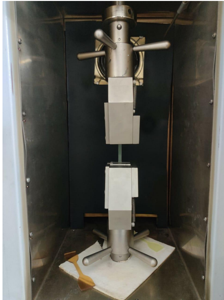
Figure 15: PU been tested in a heating chamber.
