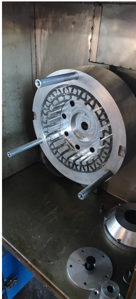
Figure 49: Mould on alignment rods in spinning oven.
