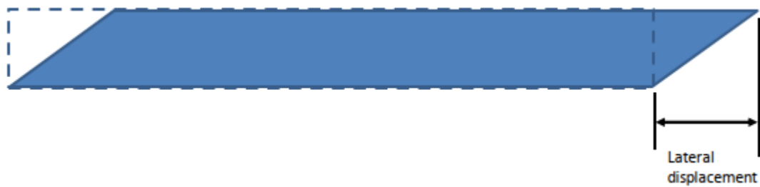
Figure 18: To achieve a shear stress in the perpendicular lateral direction, strain is applied on the lateral displacement of the clamping jaws therefore creating displacement perpendicular to the lateral.
