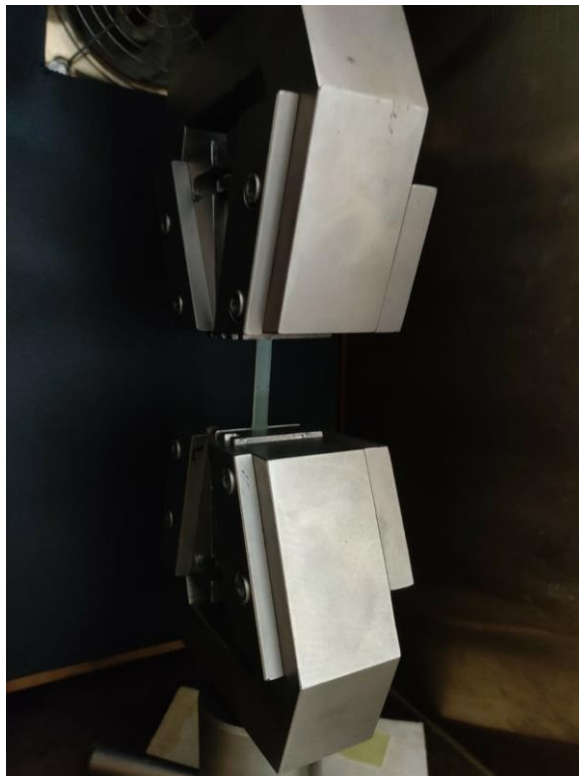
Figure 14: PU sample been tensile tested.
