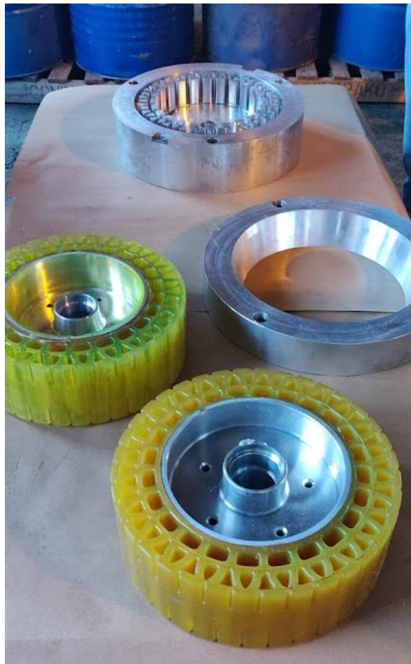
Figure 50: PU wheels cast next to the mould.
