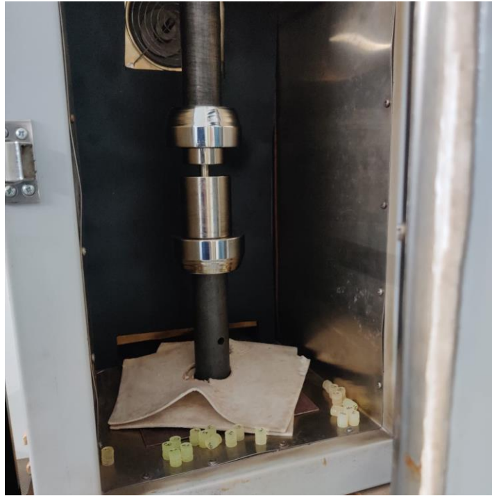
Figure 16: Compression testing of PU sample.
