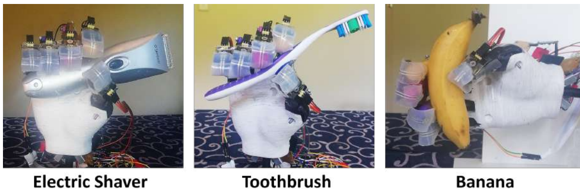
Figure 7.6: Hand Gripping Irregularly Shaped Objects
