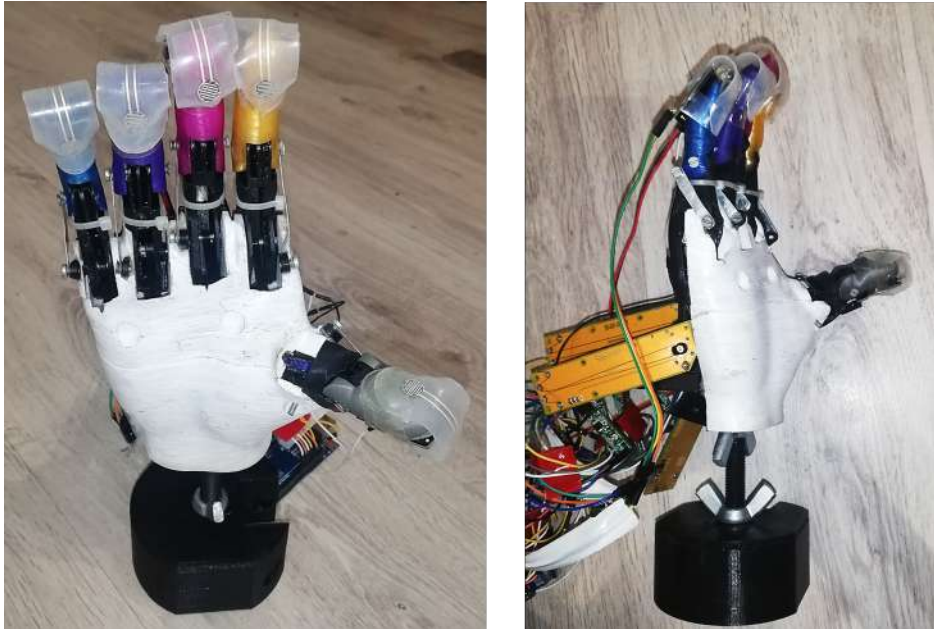
Figure 4.5: Prosthetic Hand Outfitted with Finger Pad Sensors
