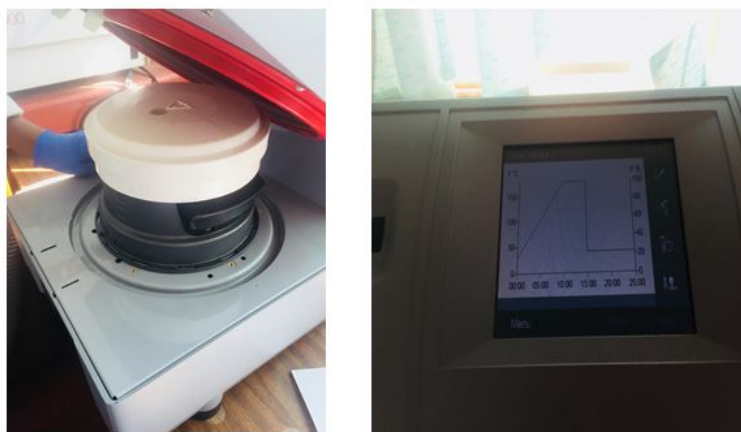
Figure 3.8: Microwave system used for sample preparation
