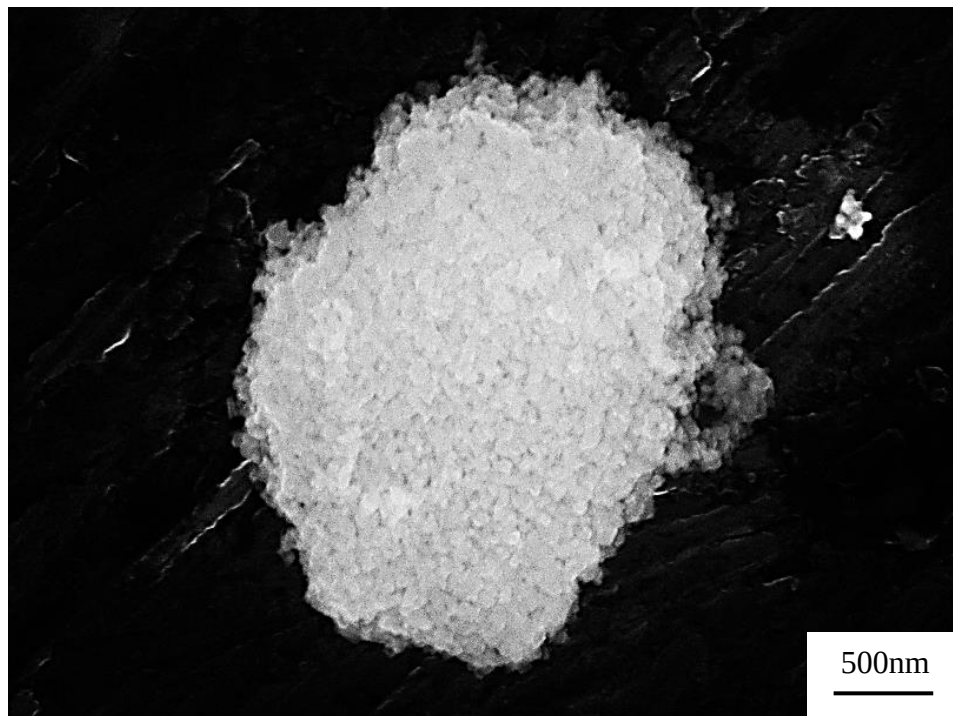
Figure 4.45: Immersion-lens SEM micrograph of the spinel powder.
