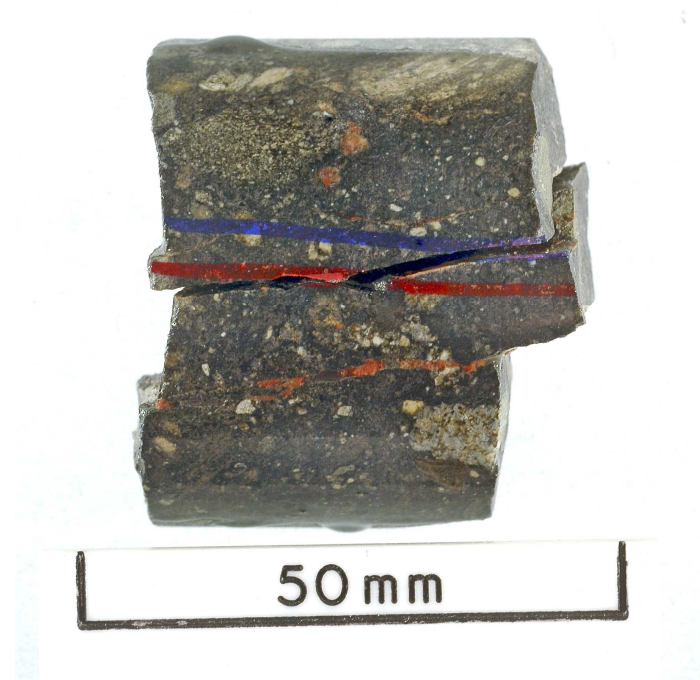
Sample RG15, Impact melt rock, 1405.25 m. A) front view, B) back view.
