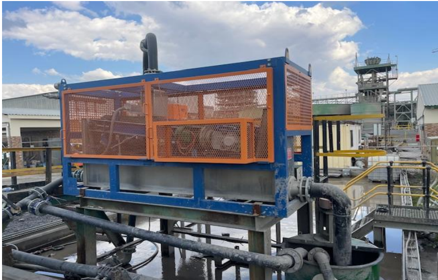
Figure 5.3 L300 WHIMS used for the test-work.
