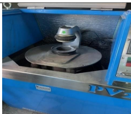
Ring Mill for pulverizing samples for wet chemical assay
