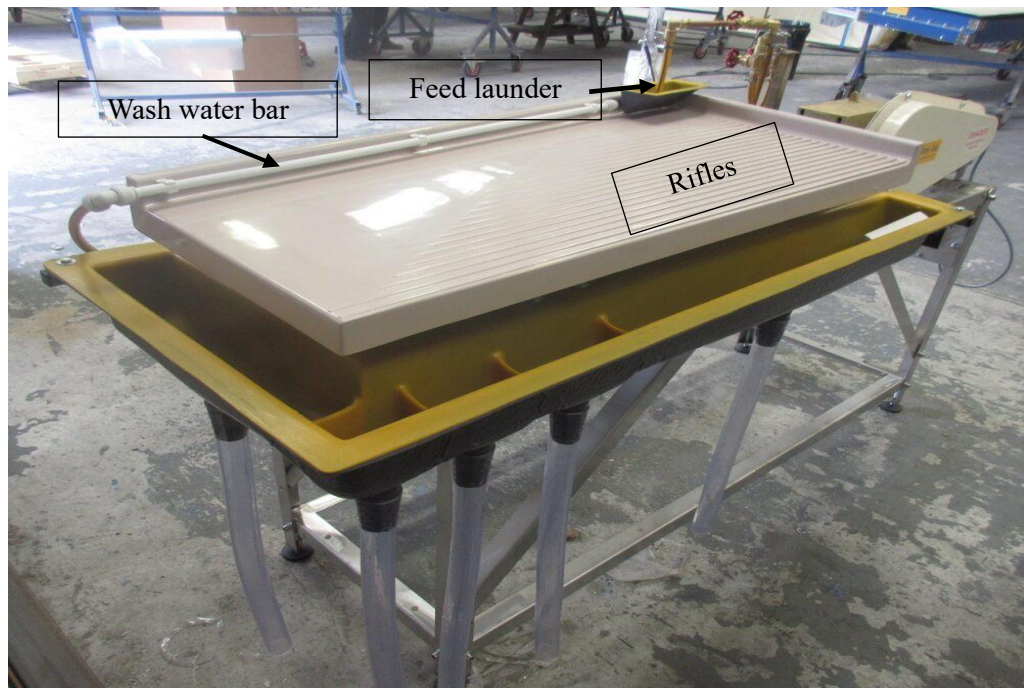
Figure 5.4 Holman-Wilfley Shaking Table Model 800 used for the test-work.
