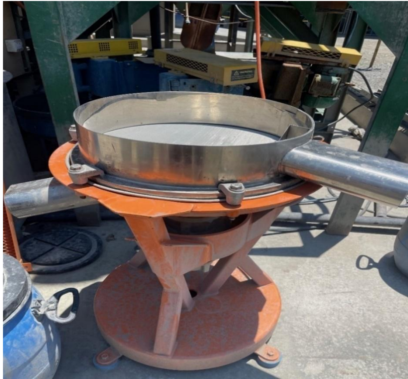
Figure 5.5 The Rhologan MK5 screen used to screen feed and product material.
