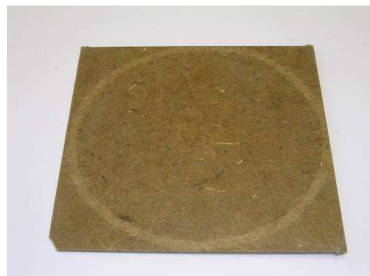
Figure 4.15 Composite production failure - loss of vacuum
