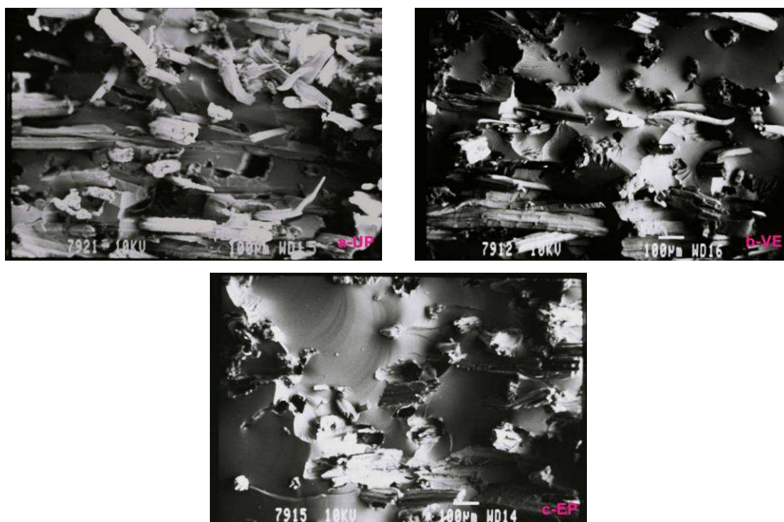
Figure E.5 SEM micrographs of impact failure surfaces of composites made using various resin systems at 22.5 % fibre volume fraction
