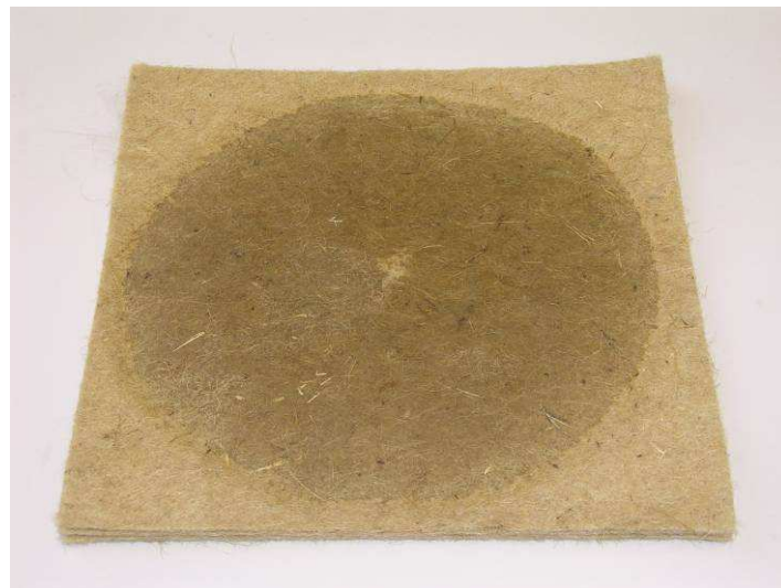
Figure 4.14 Composite production failure - resin curing during mould filling
