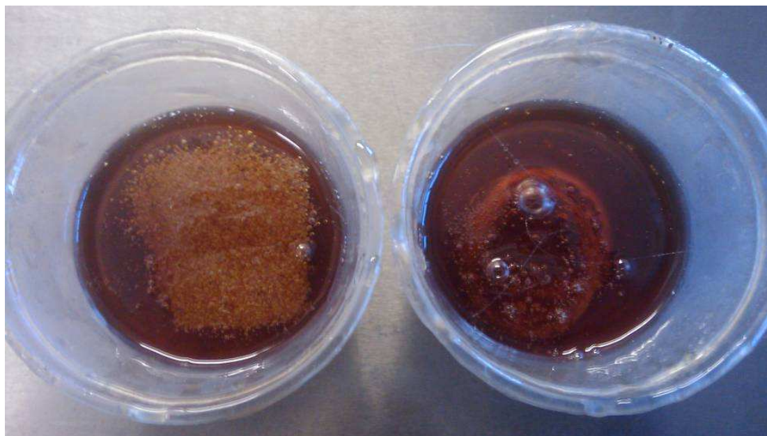
Figure 4.13 Vinyl ester resin gassing with CSM glass (left) and UD glass (right)
