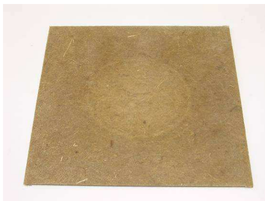
Figure 4.15 Composite production failure - loss of vacuum
