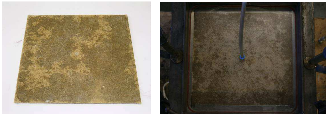
Figure 4.12 Failed vinyl ester resin composite (left) and vinyl ester resin gassing following injection (right)
