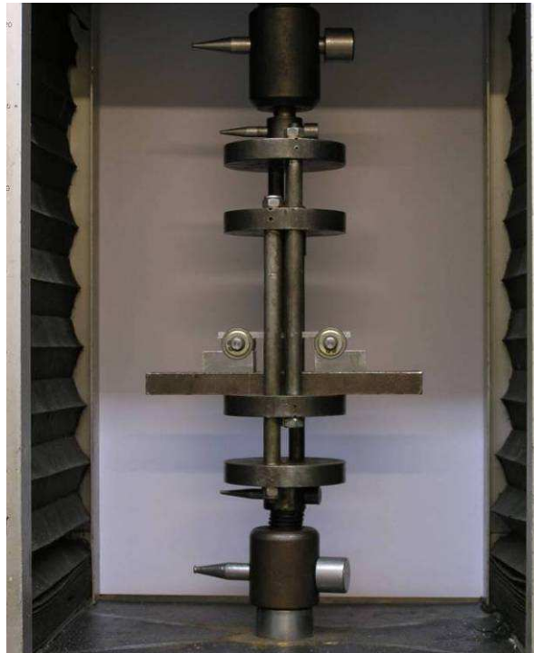
Figure 5.3 Flexural test setup
