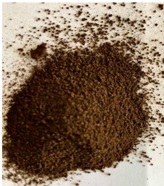
Figure 3.2 Hydrochar produced at 200 °C.
