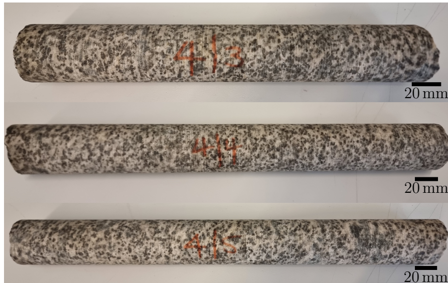
Figure 6.12: Images of the Main Zone drill cores, from the BIC, with weak remanent magnetisation. Drill cores with identifiers 4/3, 4/4, and 4/5 are presented in the top, centre, and bottom of the image, respectively. All cores had a diameter of 40 mm and cores 4/3, 4/4, and 4/5 had lengths of 290 mm, 380 mm, and 390 mm, respectively.
