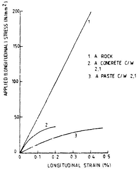
FIG 32 SCHEMATIC STRESS/STRAIN CURVES FOR ROCK, CONCRETE AND CEMENT PASTE (AFTER HOBBS<sup>6</sup>)
