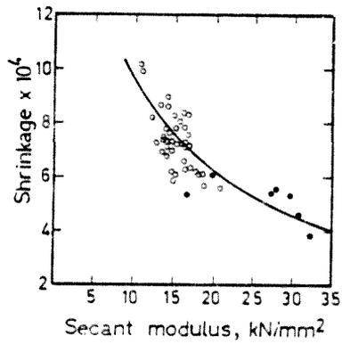
Figure 3.3 Shrinkage of Concrete Plotted Against Its Secant Modulus of Elasticity (after Reichard<sup>13</sup>)
