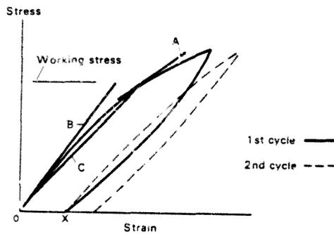
Figure 3.1 Typical Short-Term Stress/Strain Curve for Concrete (after Illston et al<sup>4</sup>)
