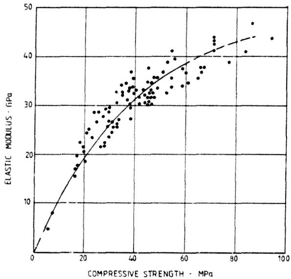
FIG 3.5 a RELATIONSHIP BETWEEN COMPRESSIVE STRENGTH
