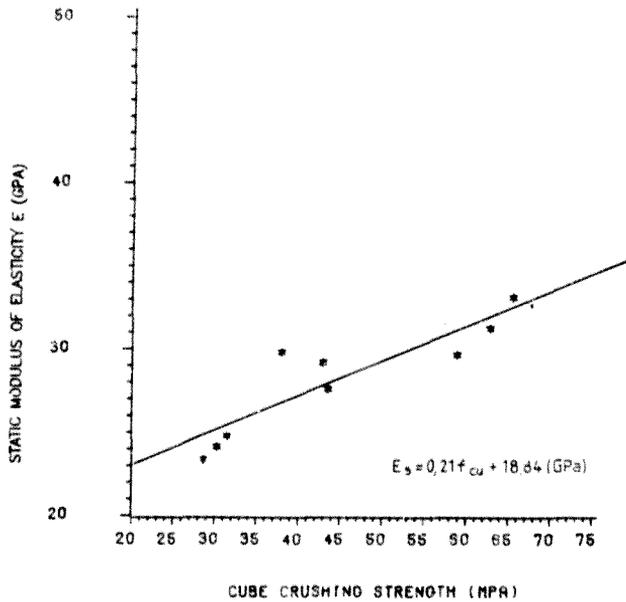
FIG 3.11a CUBE STRENGTH VS. STATIC MODULUS
