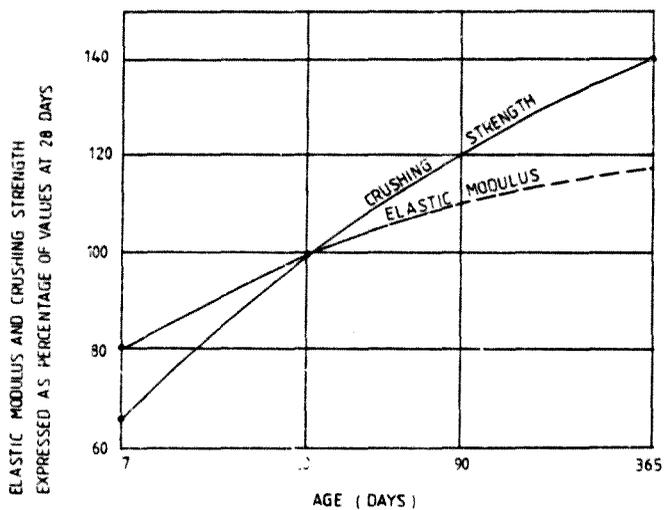
FIG 3.5b ELASTIC MODULUS AND COMPRESSIVE STRENGTH
