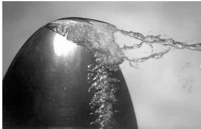
Figure 2.8: Vortex cavitation on a hydrofoil tip, an example of hydrodynamic cavitation [34].
