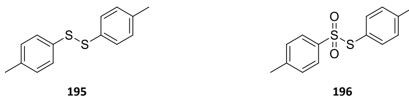
Figure 83 – An example of the disulfides and thiosulfonates generated when thiols are exposed to CAN
