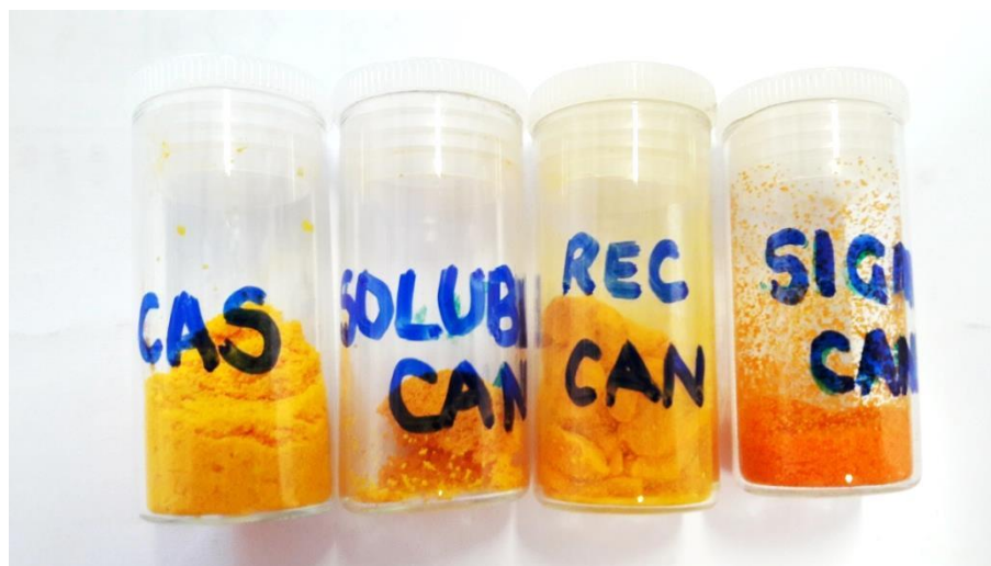
Figure 102 – Ceric ammonium sulfate, the water soluble portion of the 'Old CAN', recrystallized CAN and ceric ammonium nitrate obtained from Sigma-Aldrich (left to right) showing the distinct similarities in physical properties of CAS and recrystallized CAN.
