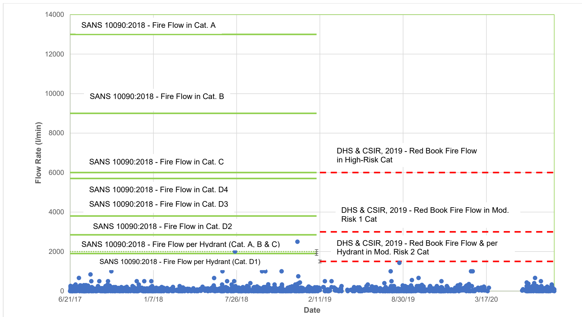
Figure 7-2 Magnitude and distribution of the fire flow rates 2060 incidents with SANS 10090 (SABS, 2018a) & Red book (DHS & CSIR, 2019) minimum flow superimposed.
