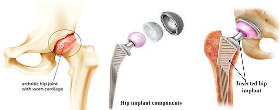
Figure 2.2: Total hip arthroplasty for an arthritic hip https://orthoinfo.aaos.org/en/treatment/total-hip-replacement/
