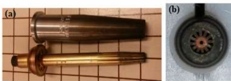
Figure 19. Two-piece oxy-fuel cutting nozzle - (a) two pieces (b) nozzle assembly (Pond & Martin, 2020).
