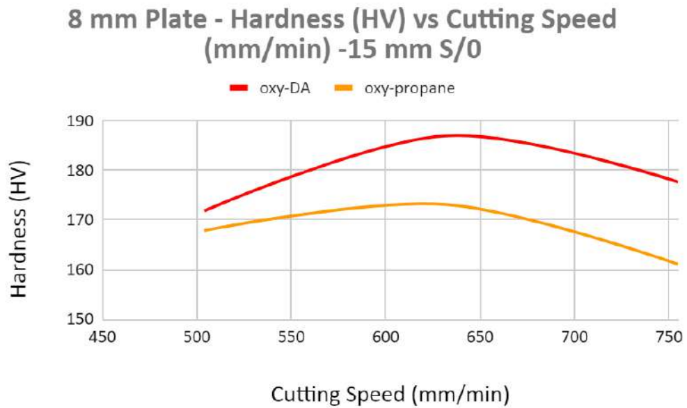
Figure 48. Variation of hardness with cutting speed for 8 mm mild steel plate at 6mm nozzle standoff (a) and 15mm nozzle standoff (b)
