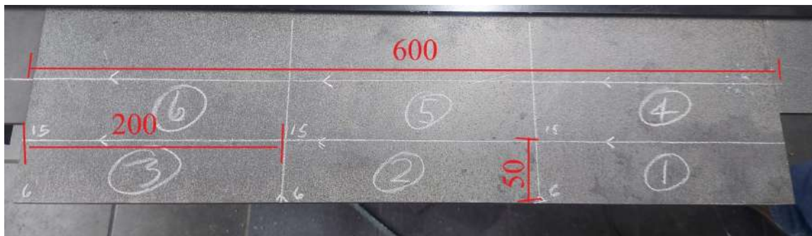
Figure 42. Sample preparation example for 8 mm thick plate for the 6 mm (No 1-3) and 15mm (No. 4 - 6) nozzle standoff
