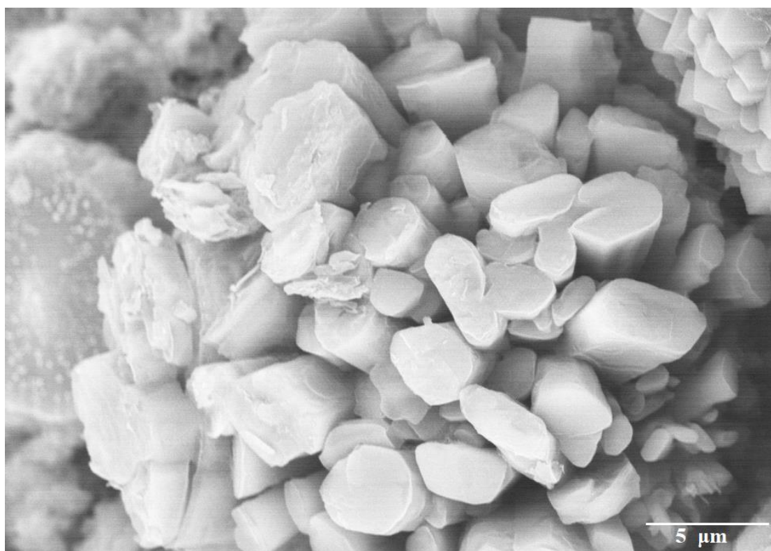
Figure 3.13 SEM image showing h-BN aggregates from CVD (900 °C)
