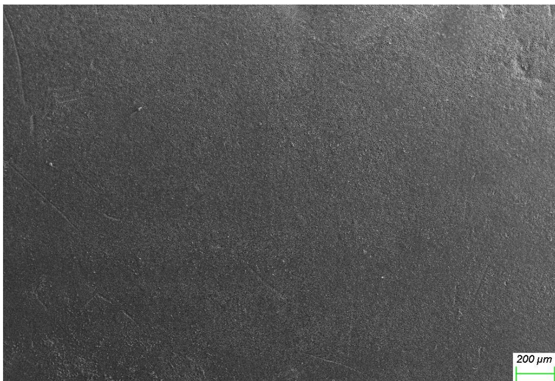
Figure B.5 SEM image of PPSU-CBN (0.8wt.%) membrane
