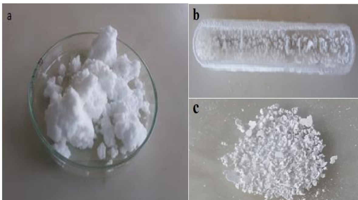
Figure 3.8 (a) Precursor formed from Boric acid and urea reaction mixture, (b) h-BN product after heating in a CVD reactor, and (c) h-BN from HTF
