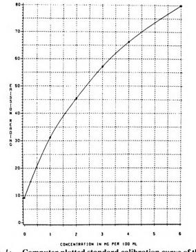
*Fig. 1:* Computer plotted standard calibration curve of the flame photometer.
