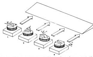
*Fig. 4:* Diagram showing the block orientations to the knife edge and direction of cuts.
