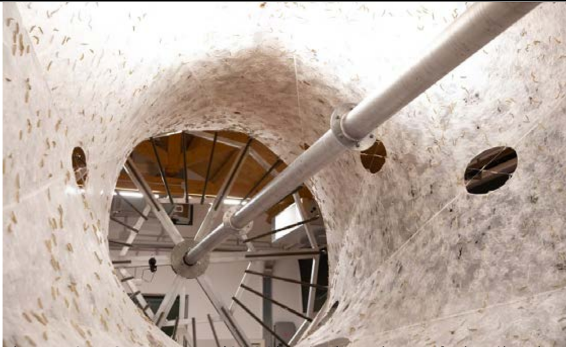
Figure 24: Oxman, N (2020) Interior View of Kinetic Jig, Soluble Knit and Live Silkworms in the Spinning Phase, Massachusetts: Massachusetts Institute of Technology.
