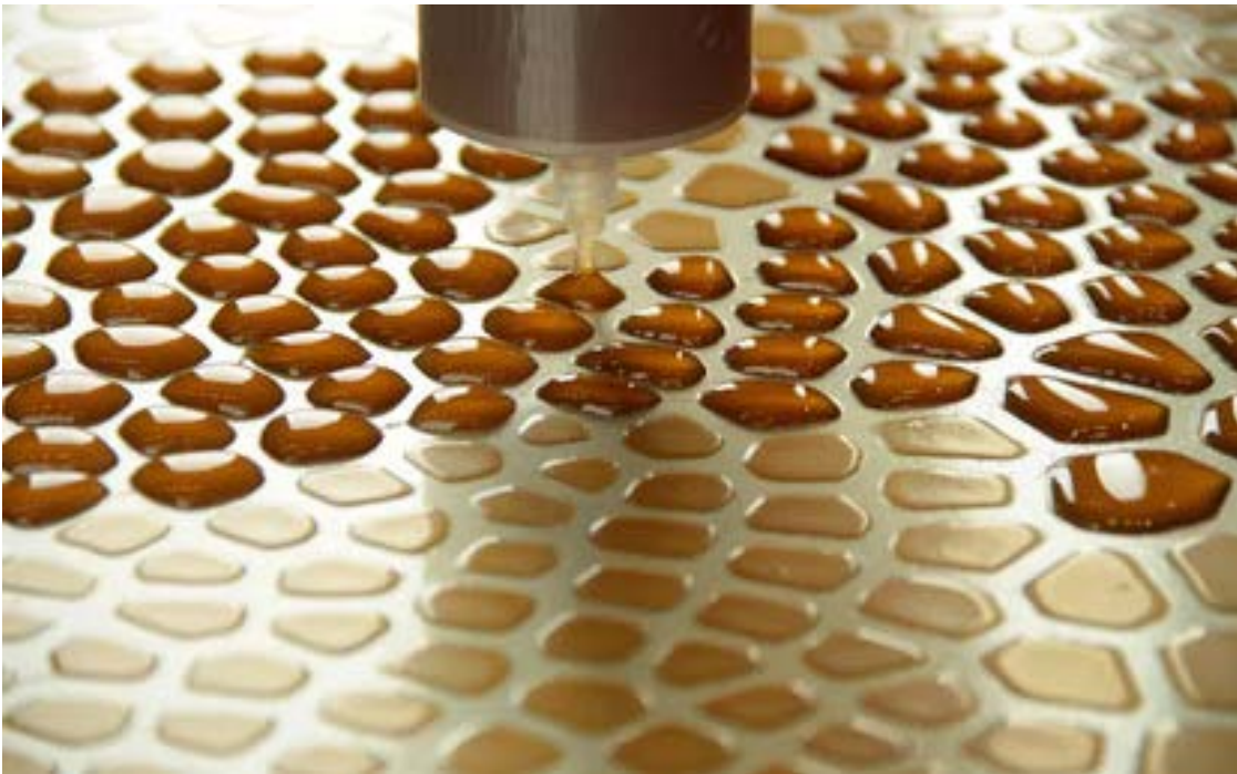
Figure 20: Oxman, N (2014-2020) Chitosan-Based Cellular Network. Colour Indicates Property Variations, Massachusetts: Massachusetts Institute of Technology.
