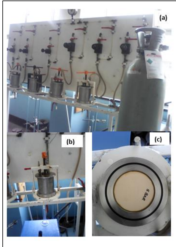
Figure 3.1: Fluid loss equipment with air cylinder (a), graduated cylinder (b) used for filtrate collection and the 5 bar ceramic disc (c) for the cell used (Civil Engineering Soil laboratory, University of the Witwatersrand, South Africa)
