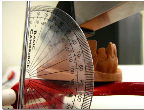
Fig 3.8 Positioning for angle for Roll
