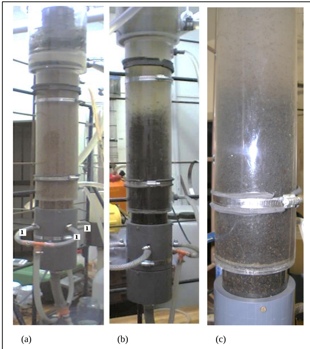
Figure 3.8: Loading of bran to bioreactor and formation of granules
