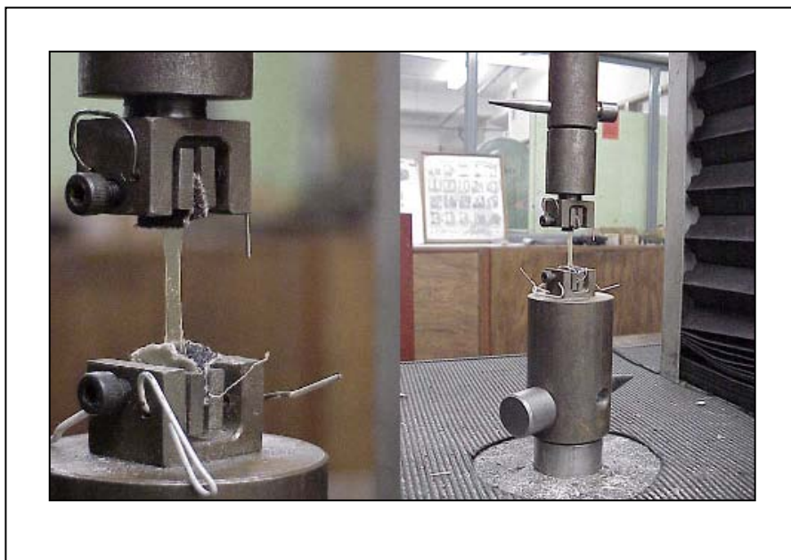
Figure 5.8 Tensile test on dog bone samples of 3mm width, 15mm long
