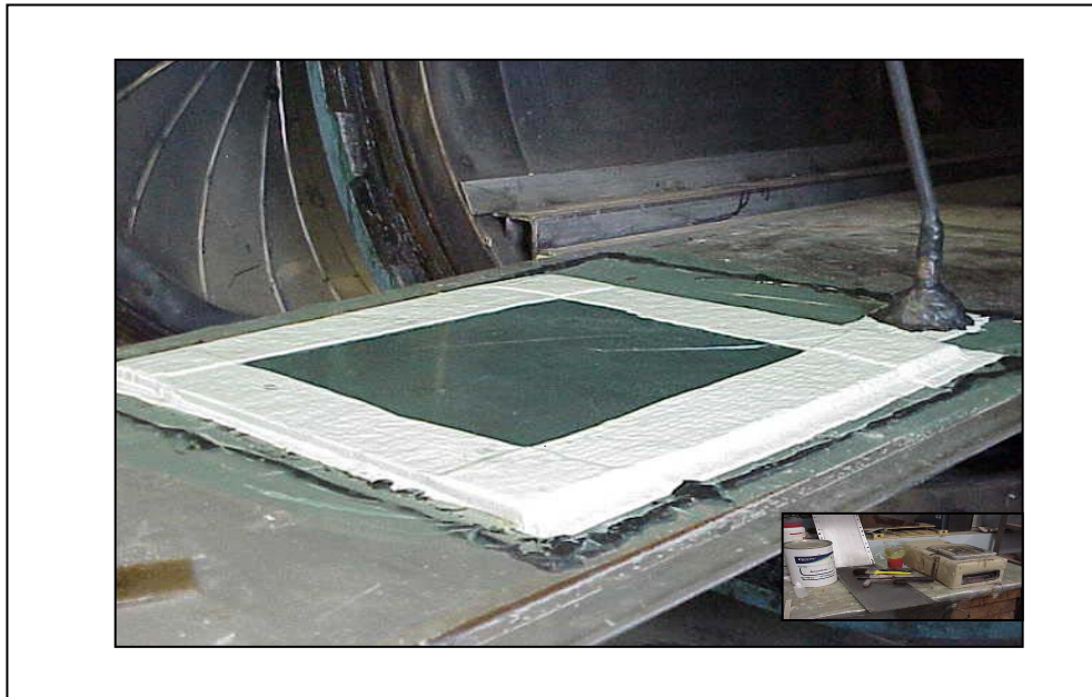
Figure 5.3 Mould compressed under vacuum bag for even resin spread
