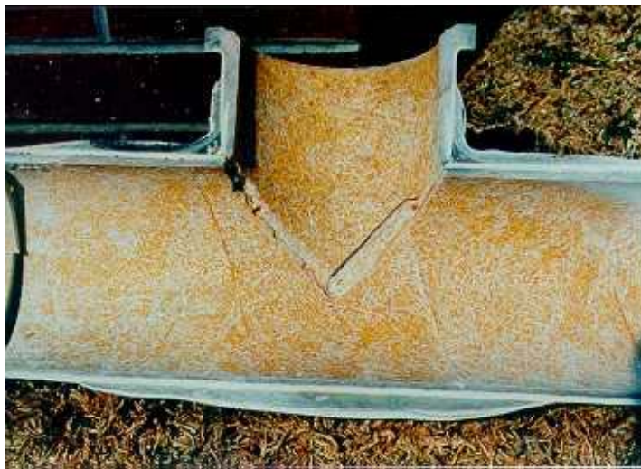
Figure 2.3 Chemical attacks on industrial pipes (with the permission of SASOL)
