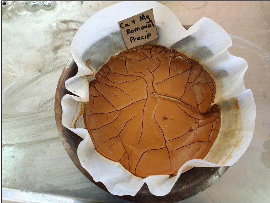
Figure 4.10: Filtered precipitate for lime-soda ash softening at ambient conditions
