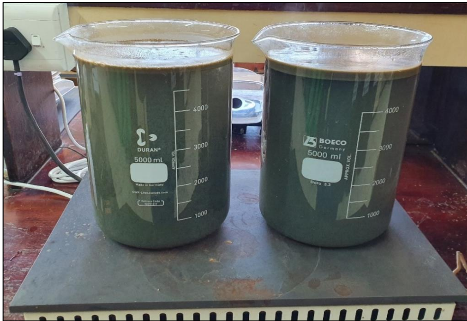
Figure 4.8: Two 5 litre glass beakers of process water treated with lime (CaO)
