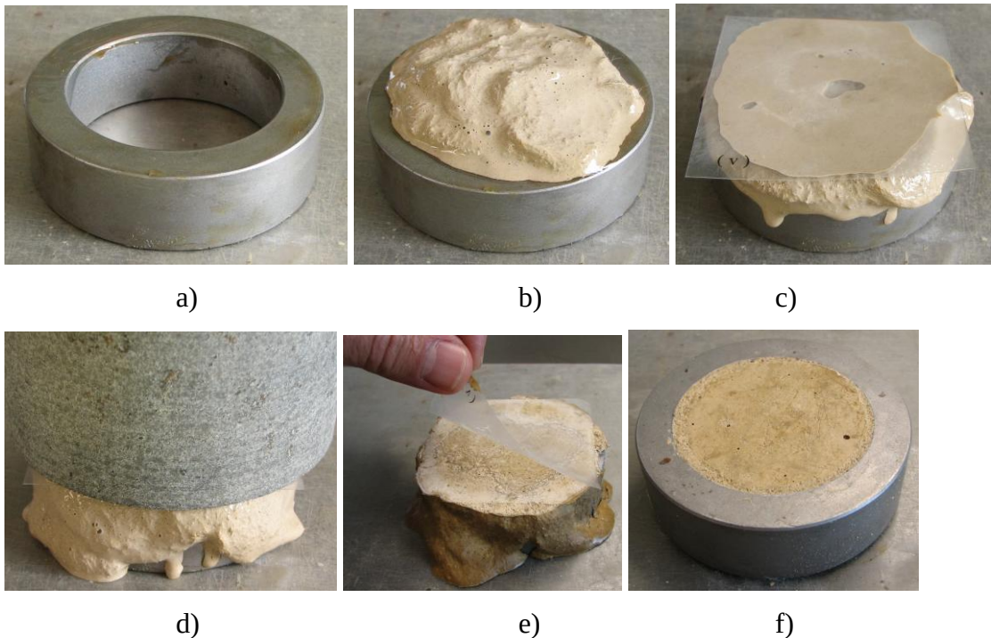
Figure 27. Steps followed during specimen preparation in material shear strength testing
