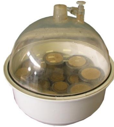
Figure 9. Water-desiccator used for the cementitious TSLs and shotcrete
