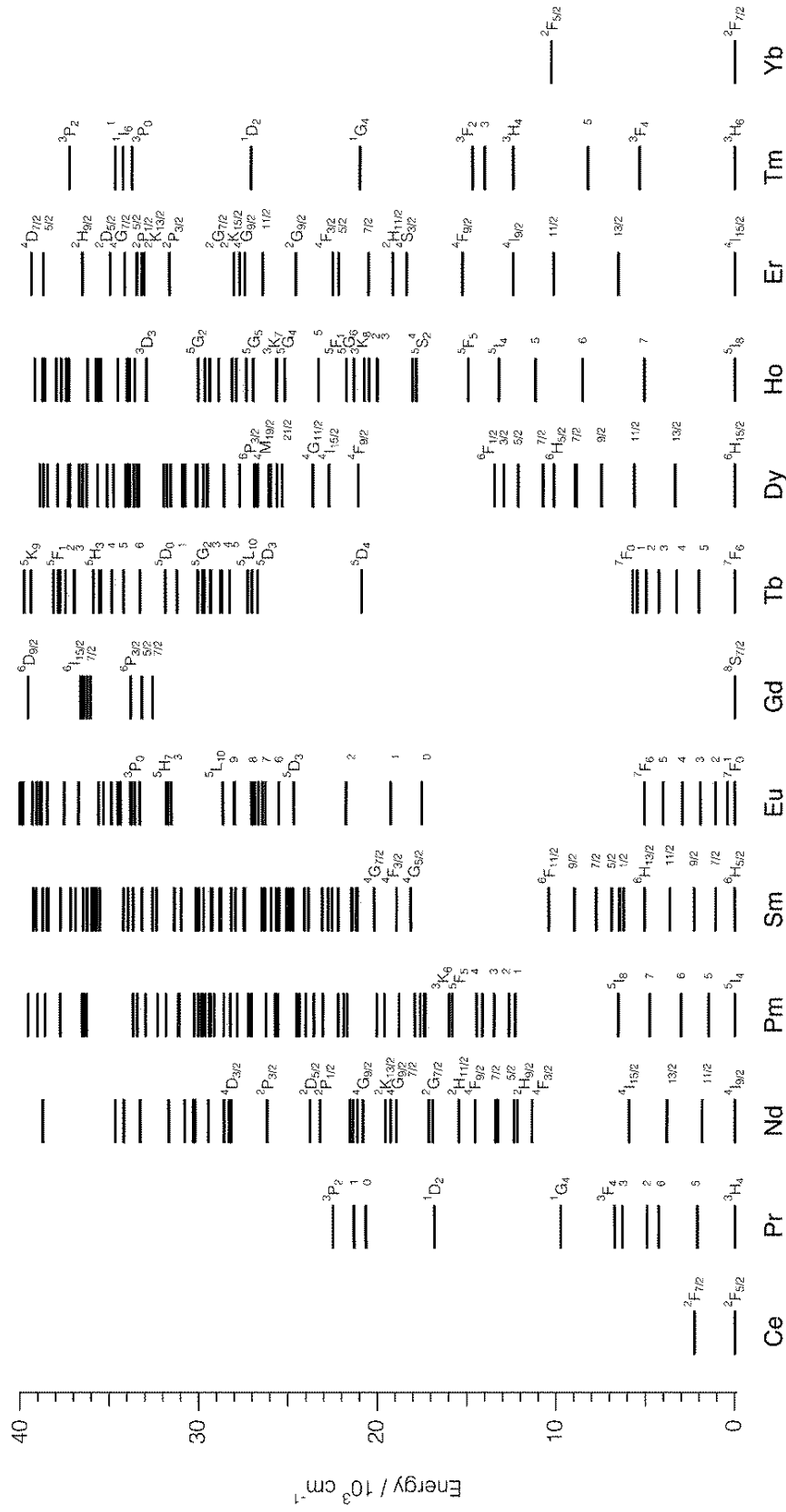
Figure 2.4: Energy levels of triply charged lanthanide ions [79]
