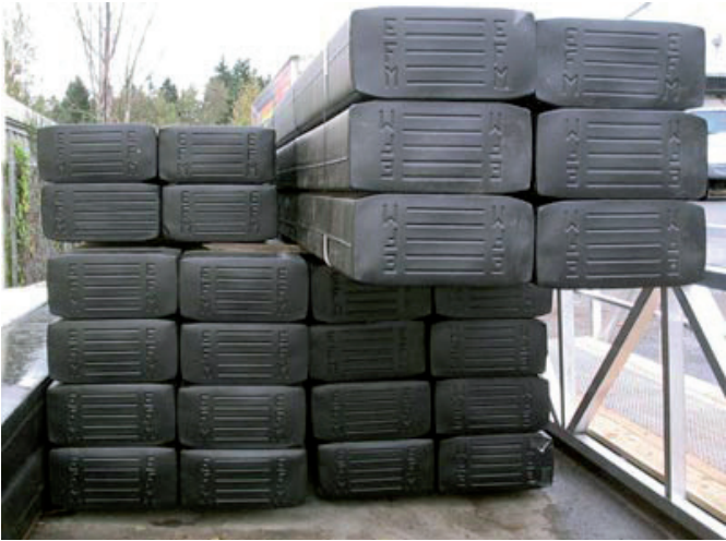
Fig 7.2.2. Hollow plastic floats used to support pontoons
