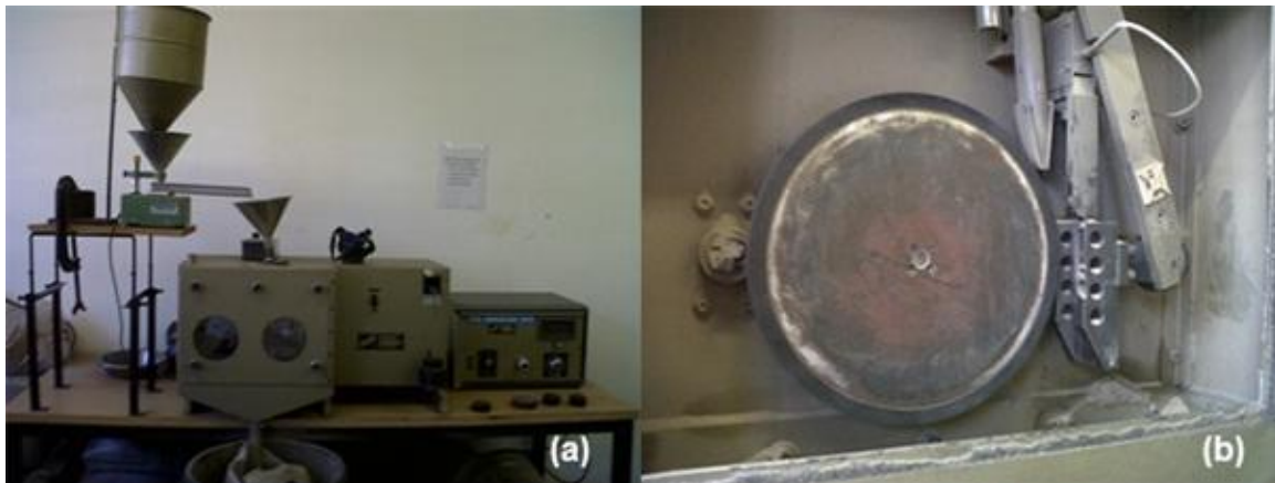
Figure 3-5: Dry sand-rubber wheel test apparatus: (a) entire apparatus and (b) rubber wheel.
