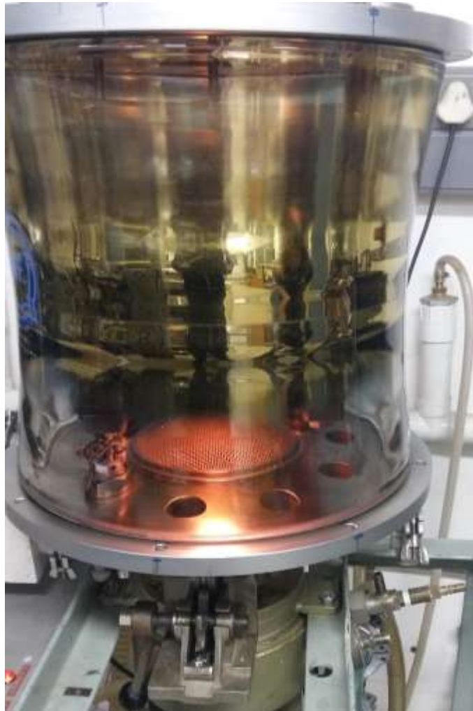
Figure S-1: Picture of thermal evaporator during Au thin films deposition in Wits.
