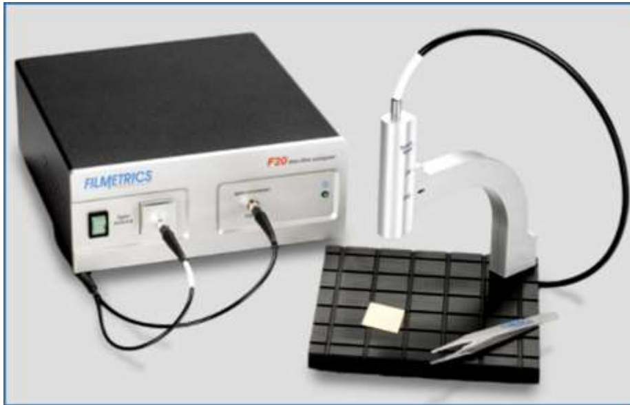
Figure 3-6: The Filmetrics F20 instrument used for thickness measurements
