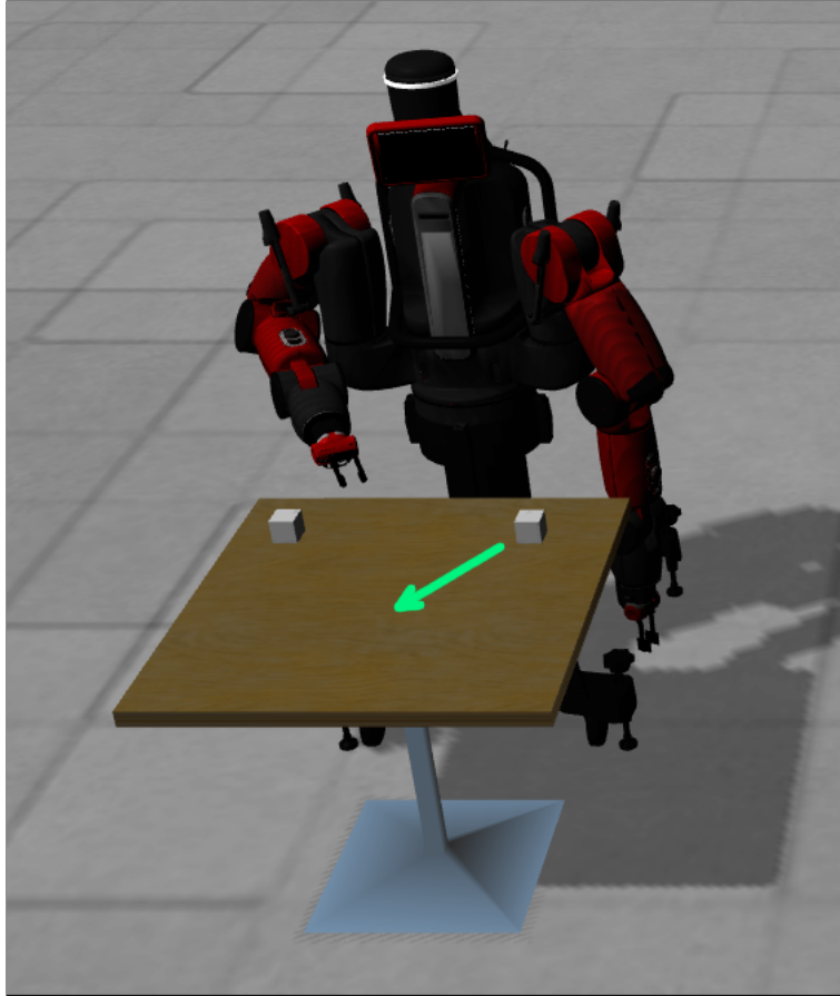
Figure 4.8: The robot arm domain. The robot alternates between picking up each of the two objects and taking them to the marked location
