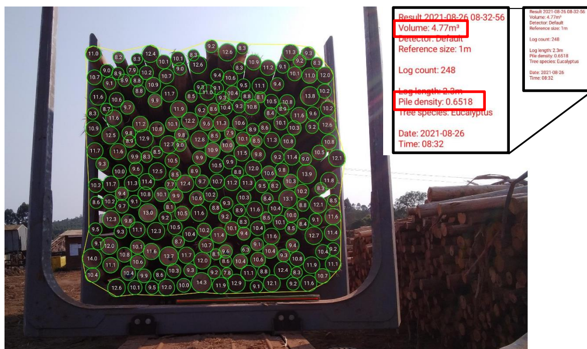
Figure 1. Timber stack density and volume measurement using Timbeter
