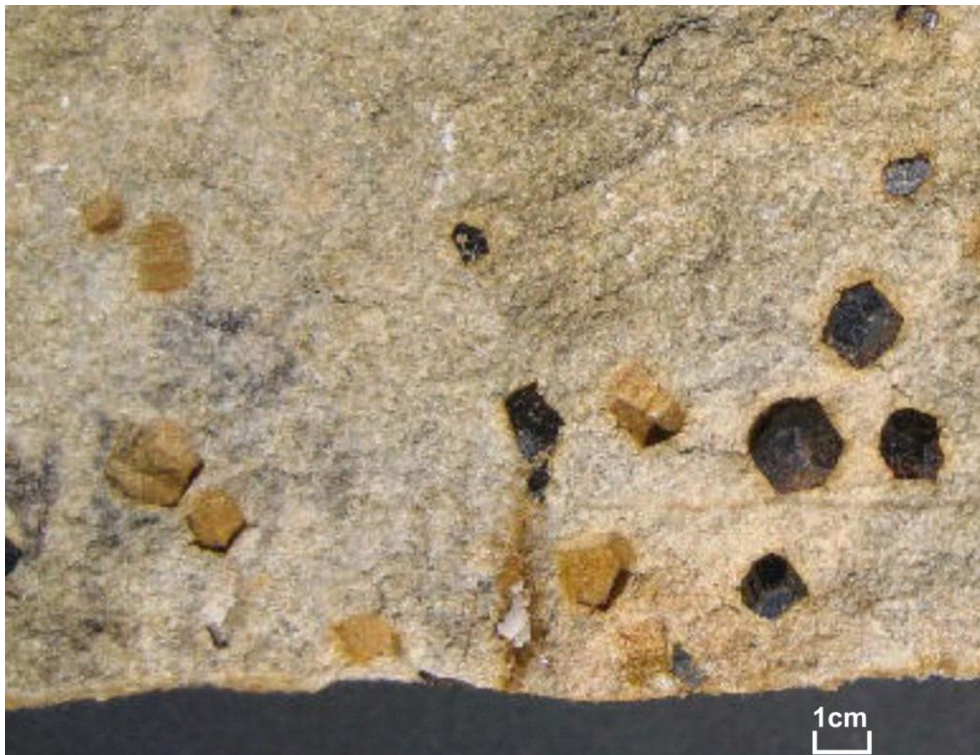
Figure 3.2: Pyrite crystals in a medium-grained sandston (arenaceous unit A)
