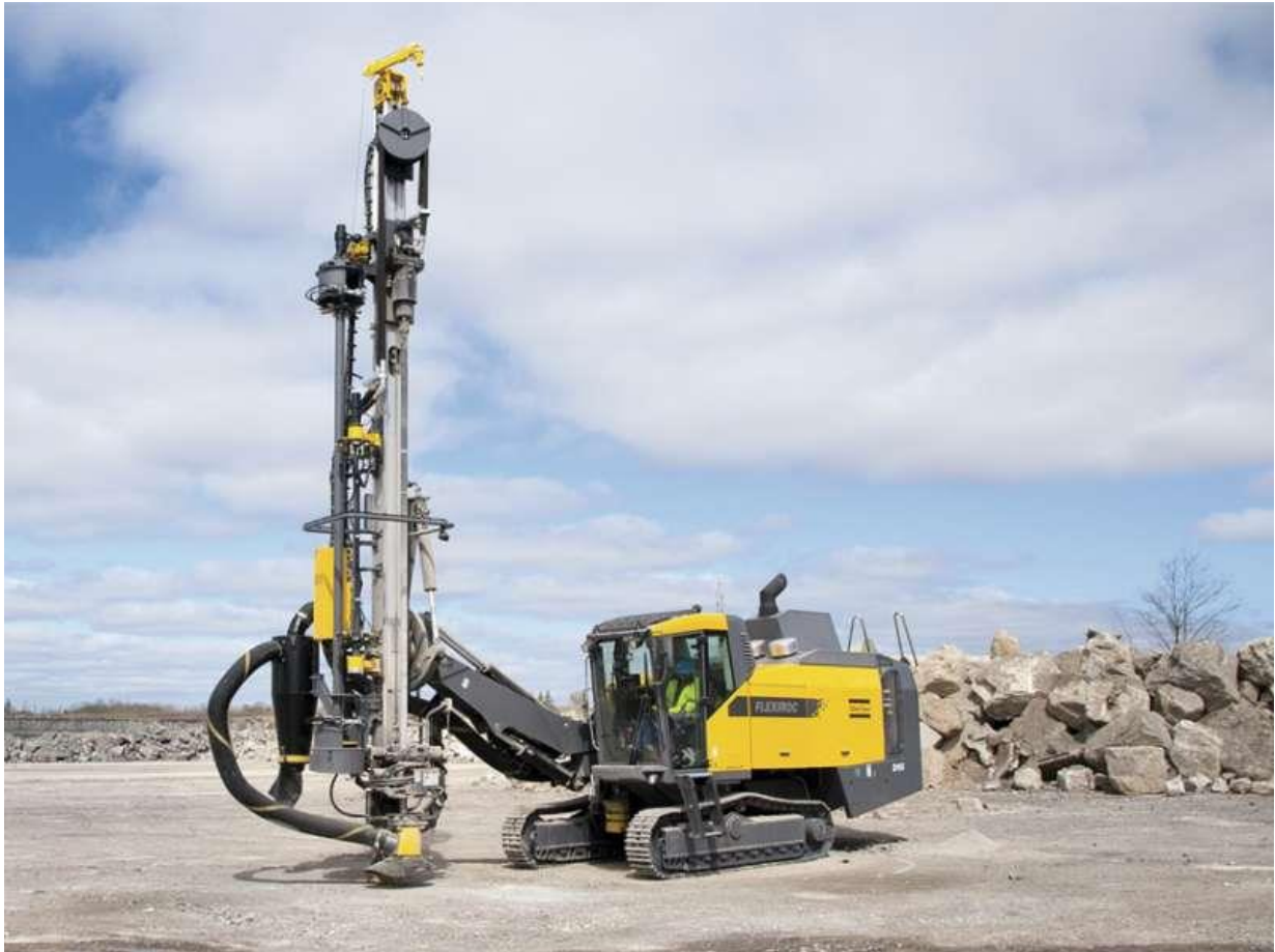
Figure 3. Drilling machine in an opencast mine (AggNet, 2022)
