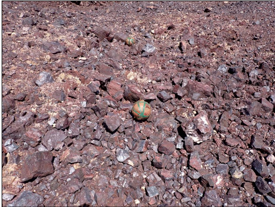
Figure 3.2: Captured image for fragmentation analysis
