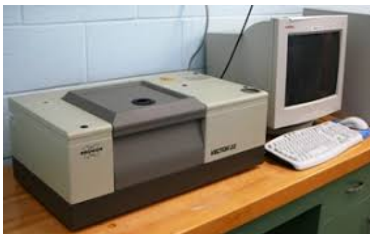
Fig 3.3 Bruker VECTOR 22 spectrometer: FT-IR analyser.
