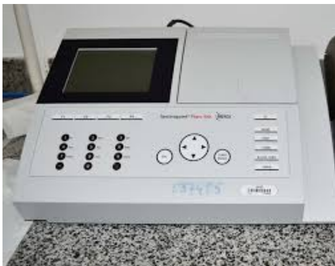
Fig 3.7 COD analysis using the UV-VIS Spectrophotometer-320.
