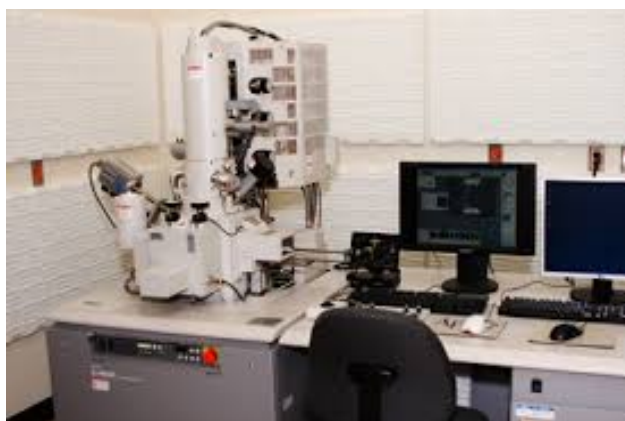
Fig 3.1 HITACHI, S-4800FESEM analyser:
