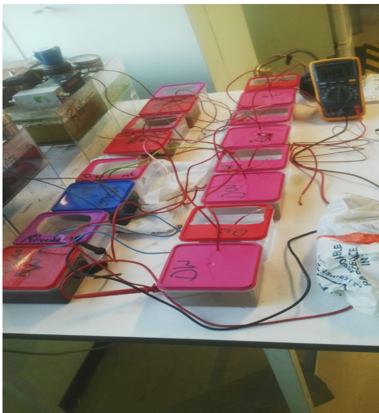
Fig 3.6 A figure showing a double chambered microbial fuel cells reactors and a Fluke 17B+ digital multimeter.
