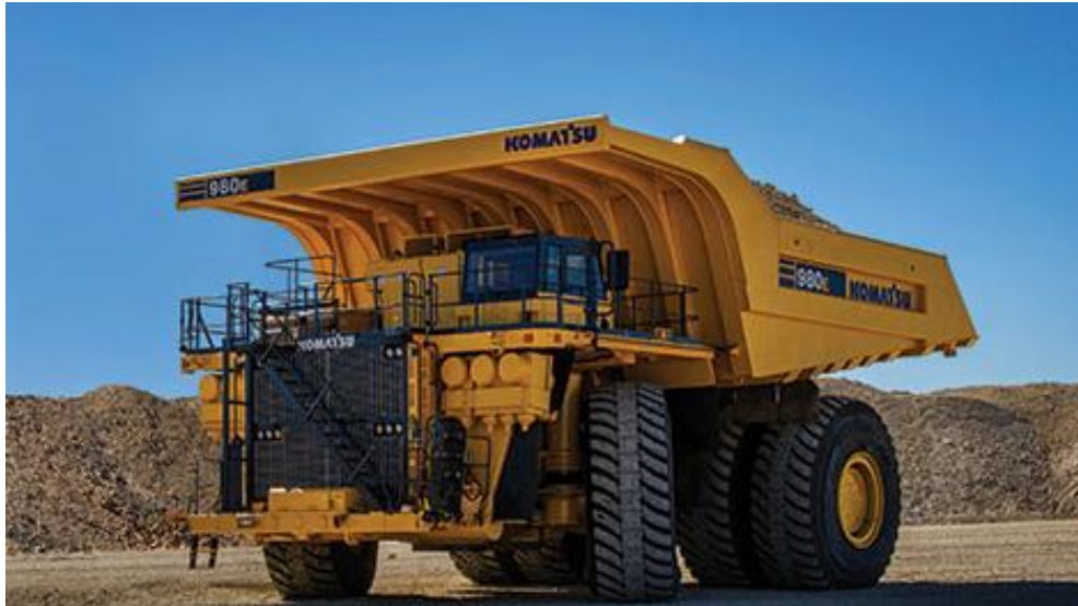
Figure 2.4: A Komatsu 980E-4 electric dump truck (Rolling Meadows, 2018)
