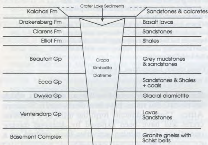
Figure 2. Generalised geological section of Orapa diamond mine.
