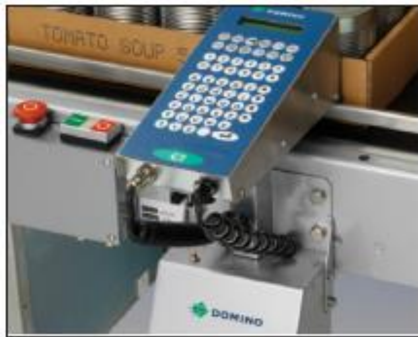
Figure 2.11 Piezo printing on a corrugate tray holding tomato soup cans (3)
