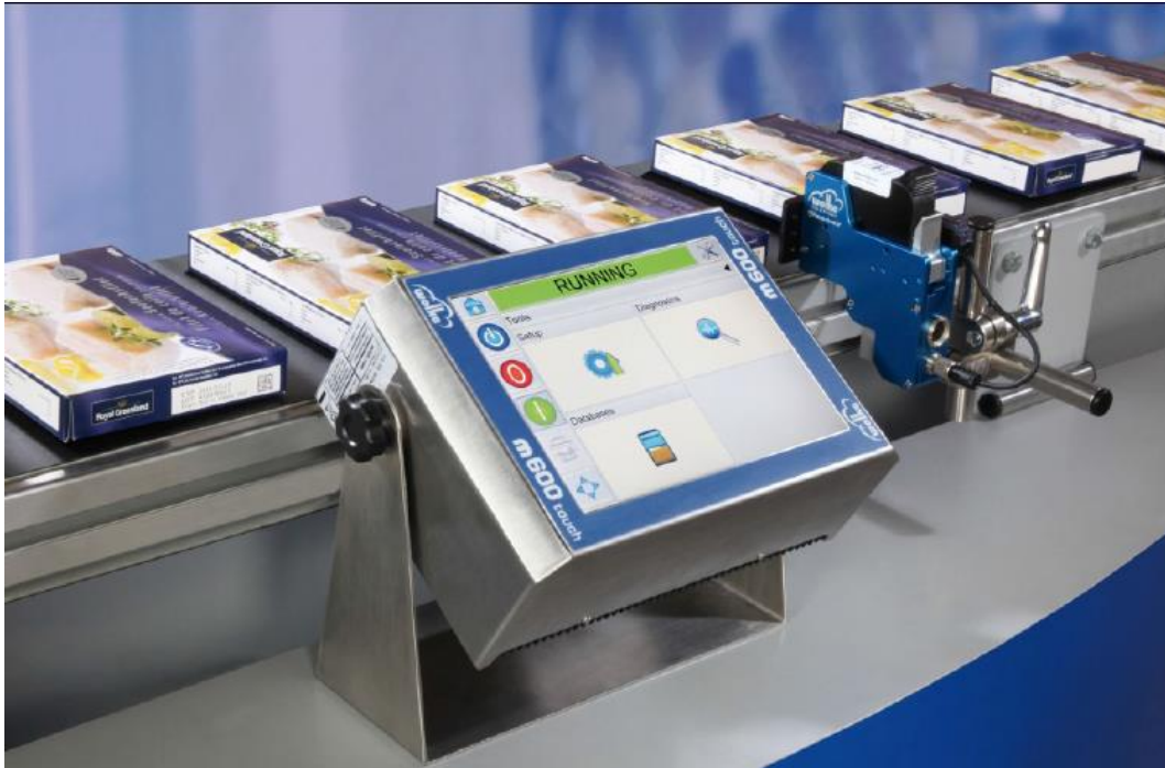
Figure 2.8 TII printing in progress on carton packaging (6)
