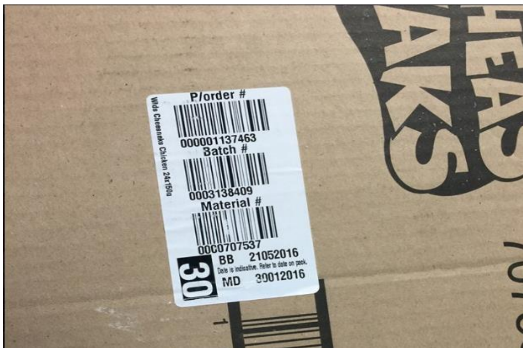
Figure 4.1 Barcode information using print-and-apply technology applied to a corrugate (28)
