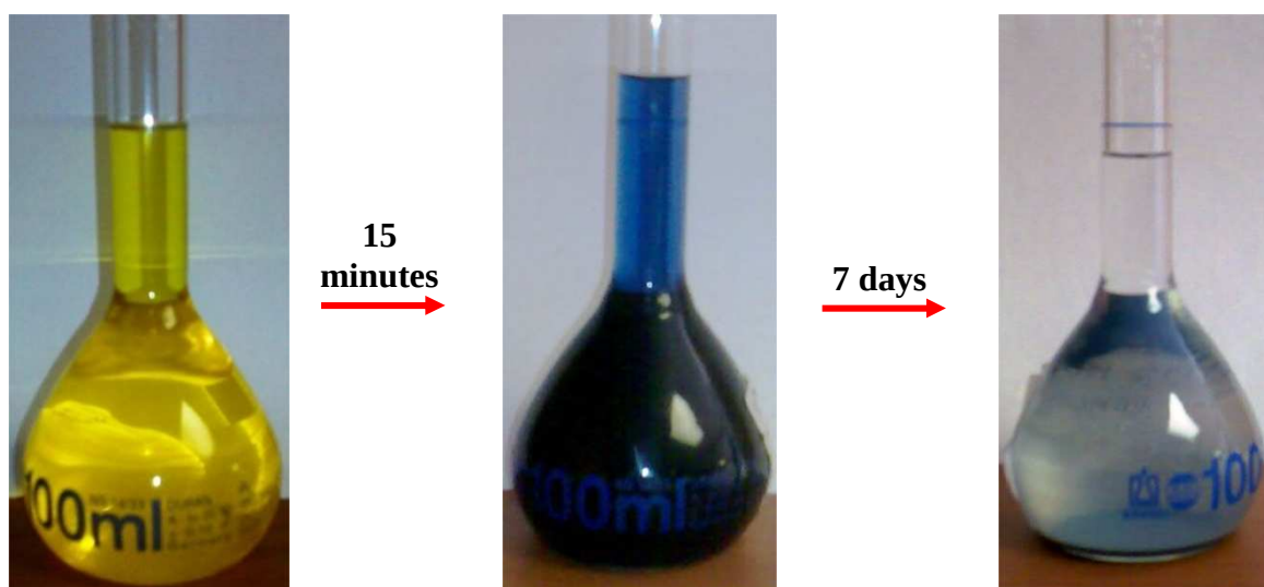
Figure 5.6 The pictures show the colour changes as the reaction proceeds to form tungsten (VI) ethoxide precursor.
