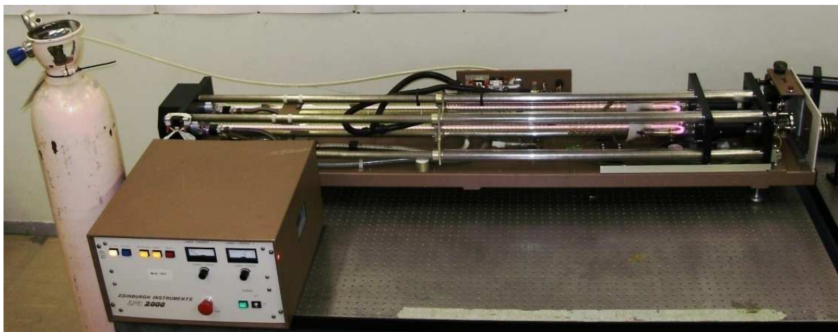
Figure 4.4 A picture of the PL6 laser, power supply and the cylinder containing the CO 2 -N 2 -He gas mixture.
