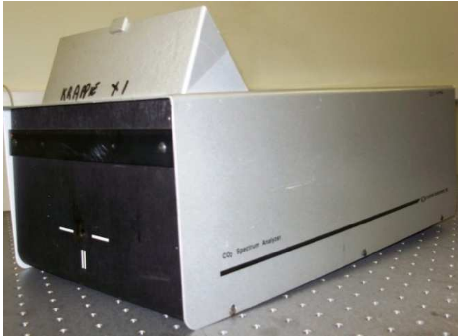
Figure 4.15 A picture of CO 2 Spectrum Analyzer (16-A) from Macken Instruments.
