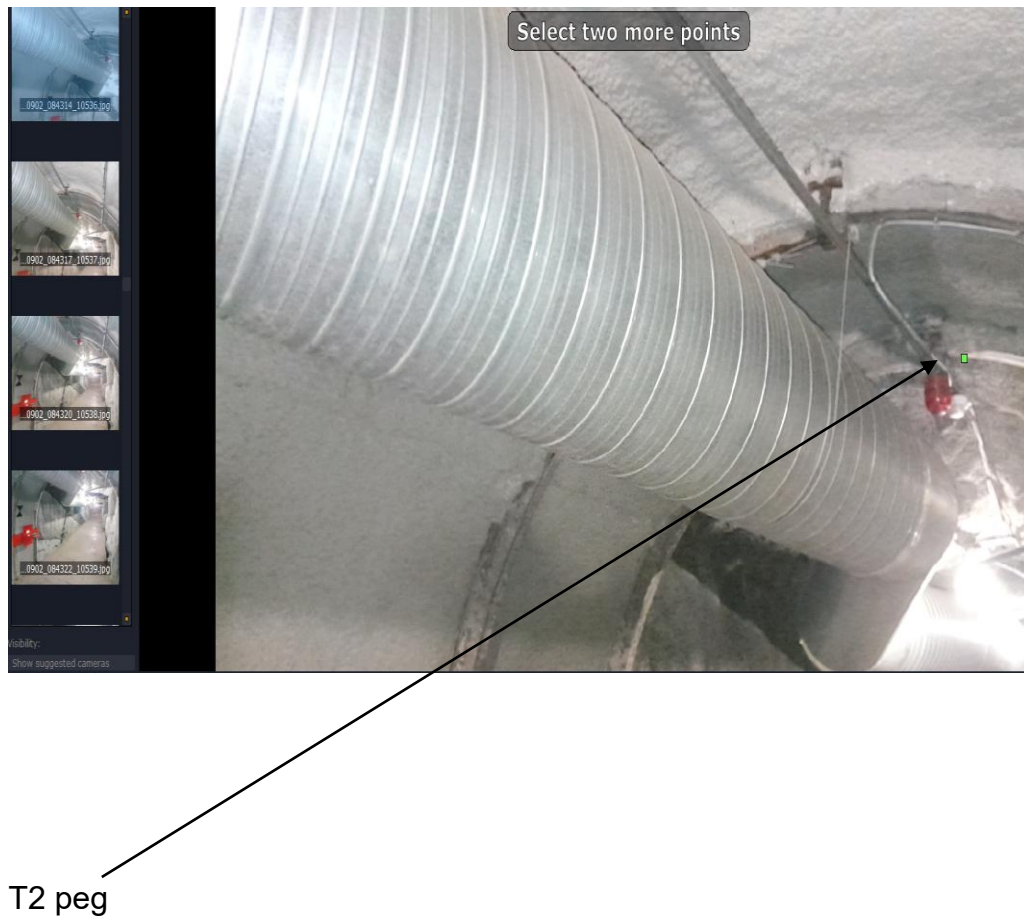
Figure 5.7: Illustration of a peg detected on an image for georeferencing of CRP 3D models.
