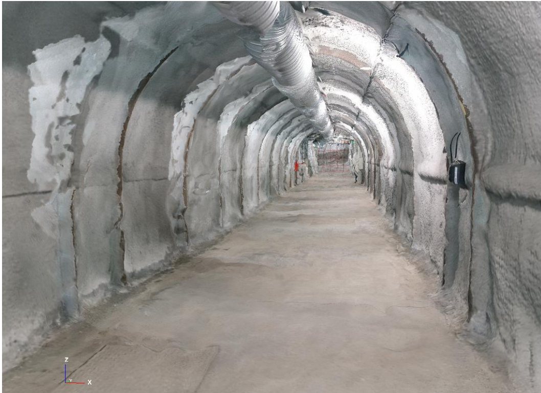
Figure 5.4: Registered point clouds in a reconstructed 3D model of the Wits Mock Mine tunnel using the CRP principle.
