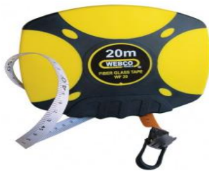
Figure 3.4: Tape measure used for conventional measurements of varying components in the Wits Mock Mine tunnel including objects indicating post-deformation properties.
