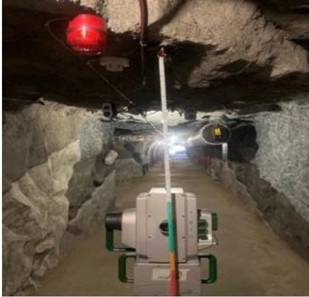
Figure 5.1: Illustration of how LiDAR was positioned under each peg in the Wits Mock Mine.
