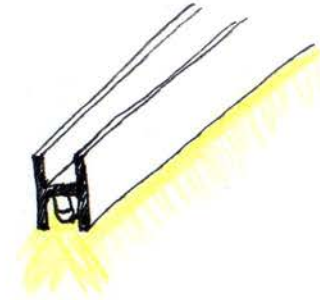
Lights hidden within structural I beams
