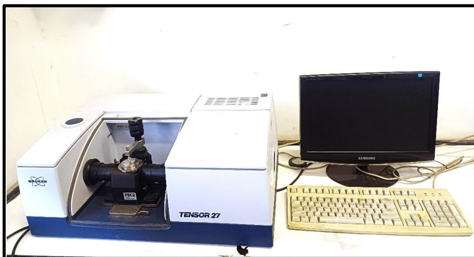
Figure 3.1: Bruker Tensor 27 FTIR instrument.
