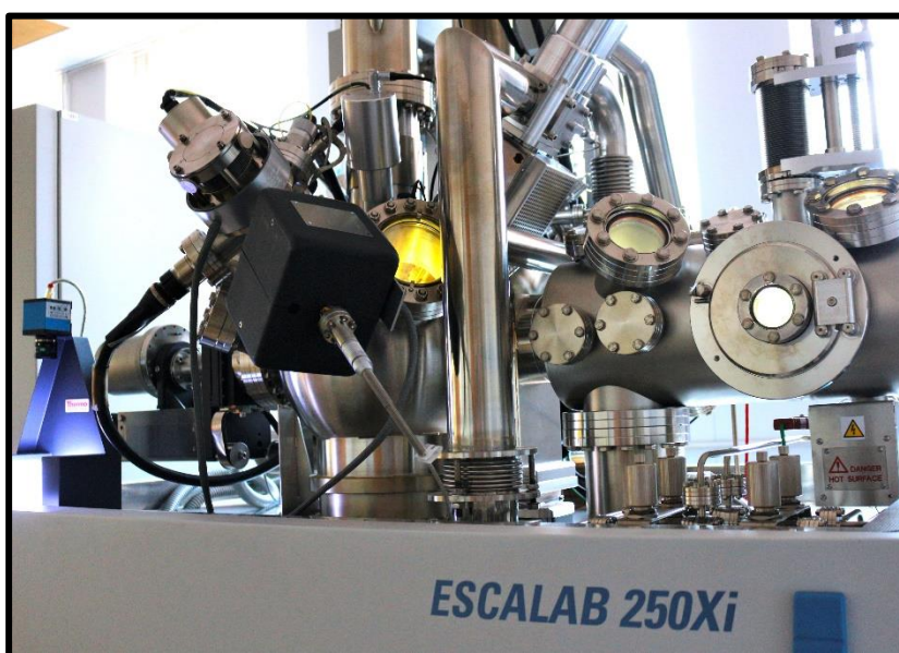
Figure 3.9: ESCALAB 250Xi XPS instrument
