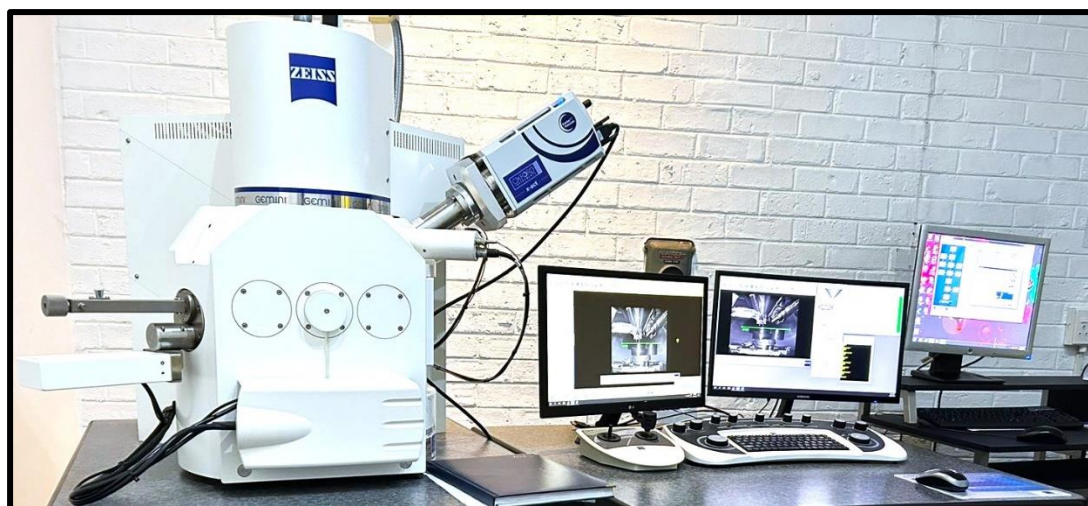
Figure 3.7: Zeiss Sigma 03-39 Fe-scanning electron microscope.
