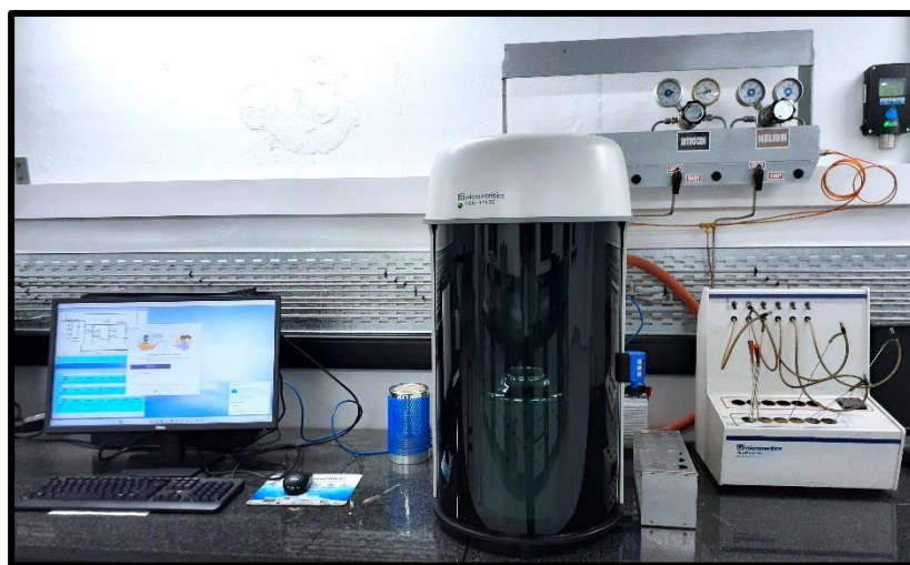
Figure 3.6: Micrometrics TriStar II plus BET instrument.
