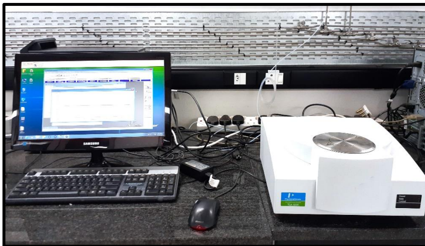
Figure 3.8: Perkin Elmer 4000 thermogravimetric analyser.
