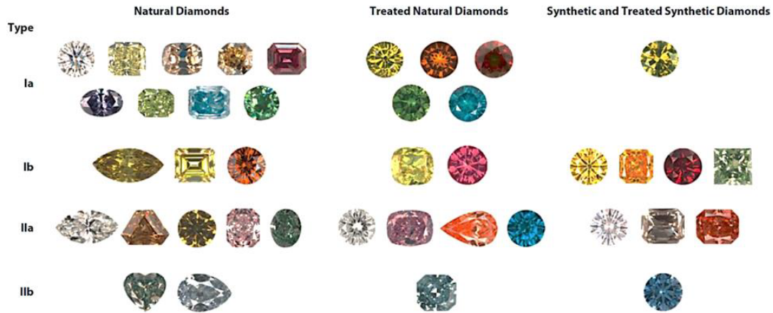
Figure 2.1: Diamond types due to defects. Four main types of diamonds that are both natural and synthetic. The different colors are due to unique impurity types and impurity levels. [45].
