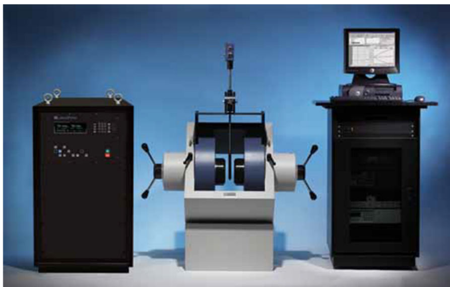
Figure 4.12: A Lake Shore transport measurement system. The system is capable of measuring the electronic transport characteristics of electrically conductive materials.
