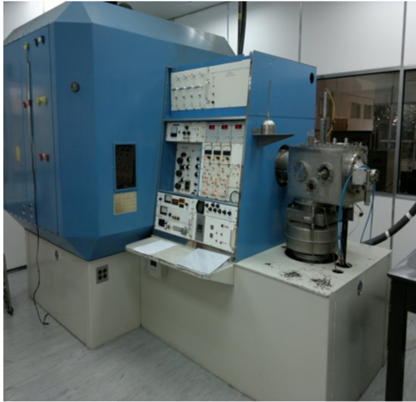
Figure 4.5: Photograph of the ion implanter at iThemba LABS. A Varian-Extrion model 200-20A2F.
