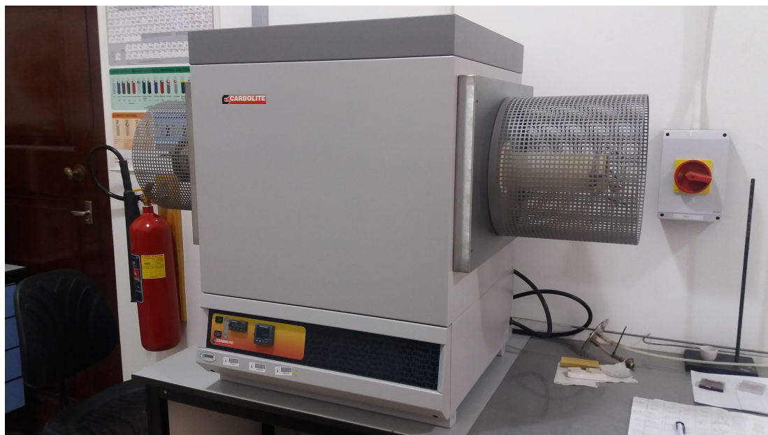
Figure 4.7: A photograph of a Carbolite high temperature horizontal thermal tube furnace. A wire wound tube furnace (CTF 17/300) with a 0°C – 1700°C temperature range.
