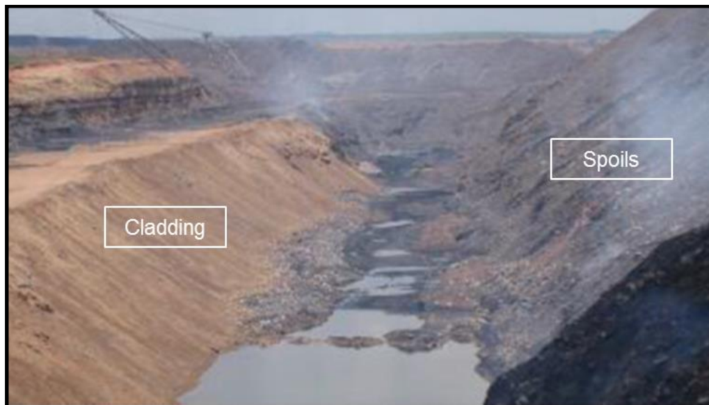
Figure 2-5: Cladding of open voids (Rogans, 2008)
