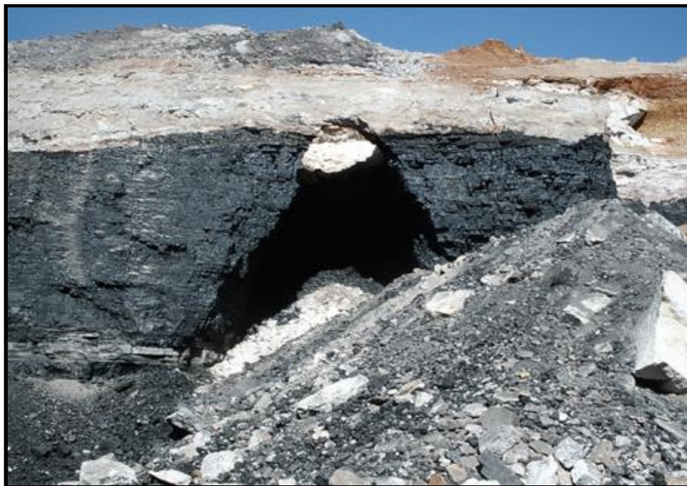
Figure 2-13: Voids that failed to collapse (Anglo American, 2012)
