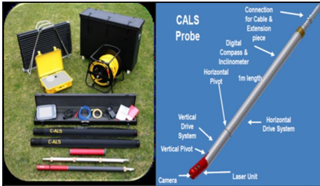
Figure 3-10: Components of a CALS Tool (Dane, 2012)
