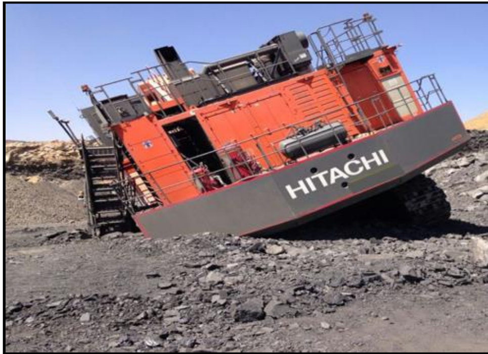
Figure 2-12: Face shovel falling into a void (Tweefontein Opencast Colliery, 2015)
