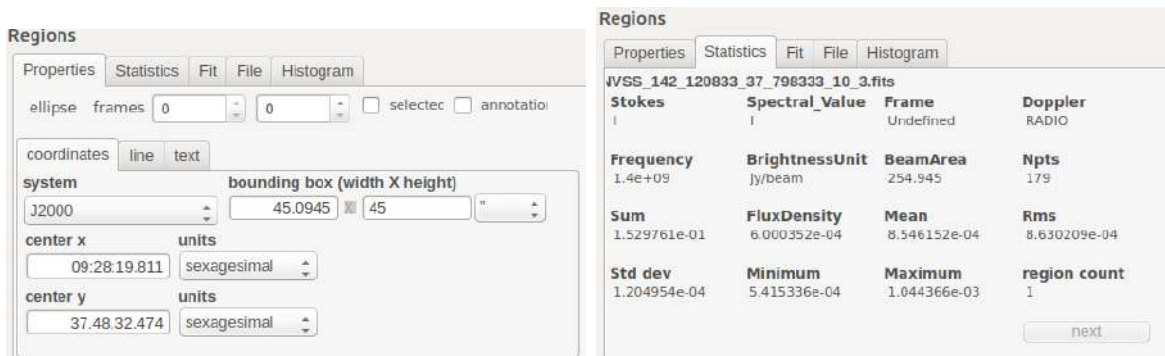
Figure 3.4: An illustration of how radio information on a specific region is obtained using the CASA interactive tool. Left: The region properties is used to define the shape, size and position of the beam we want to integrate over, right: the region statistics give the radio information of the specified area.
