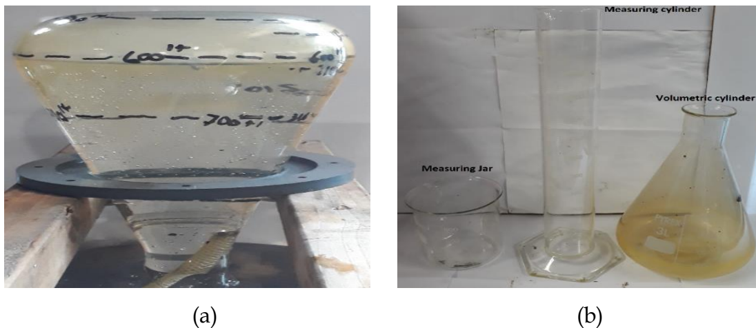
Fig 3. 5: Gas volume measuring method (a) and water volume measuring apparatus (b)
