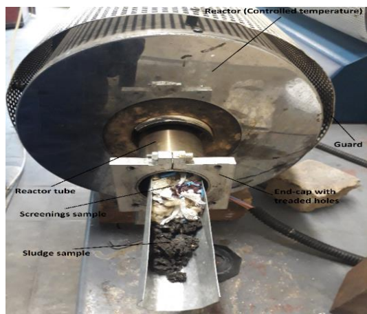
Fig 3. 4: A typical sludge and screenings sample loading in a reactor
