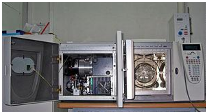
Figure 2.15 The inside of the GC-MS, with the column of the gas chromatograph in the oven on the right and the MS on the left
