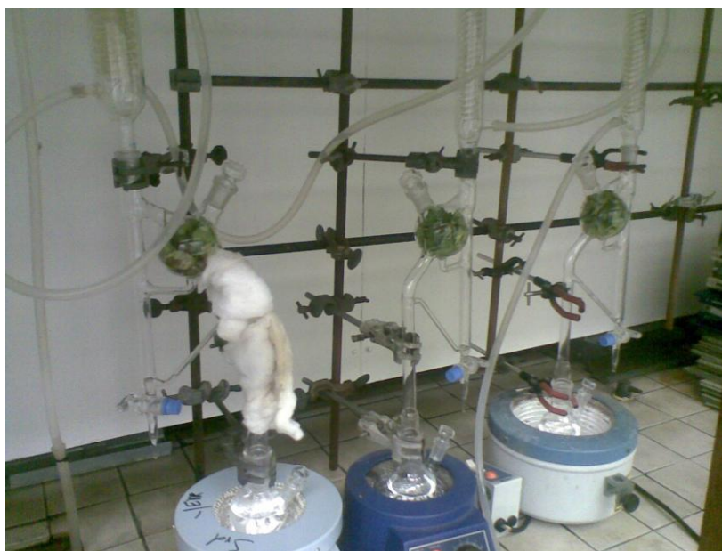
Figure 2.4 Picture to illustrate the connecting tube of the Clevenger apparatus covered in cotton wool
